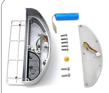
Remove the battery cover from the bottom of the light.
