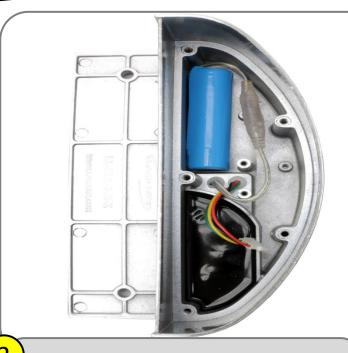
Connect battery with identical clear wire inside.
