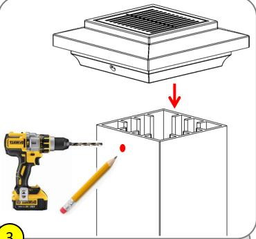
Place the solar Post Cap on the post. Mark both holes on the post. Use an appropriate drill bit to make a small pilot hole for the provided screws.
