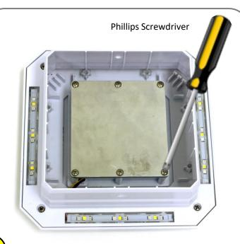
Ensure the silicone pad is under the battery cover and reinstall the cover in place. Tighten all screws to ensure a waterproof seal.
