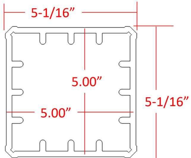
**NOTE:** TimberTech Post Covers measure approximately 5-1/16" x 5-1/16" from the protruding corners. The flat sides will measure approximately 5.00x5.00". If you have TimberTech Post covers please make sure to order the correct base adaptor.
