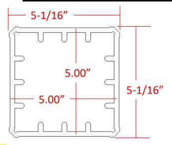
NOTE: TimberTech Post Covers measure approximately 5-1/16" x 5-1/16" from the protruding corners. The flat sides will measure approximately 5.00x5.00". If you have TimberTech Post covers please make sure to order the correct base adaptor.
