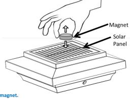
TIPS & TRICKS: If you purchased multiple units place multiple magnets together creating a stronger magnet. This will help increase the size of the activation area and allow you to activate the switch further from the light!
