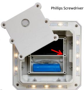
Use a screwdriver to remove the battery cover & connect the battery: NOTE: Align the connectors before joining.
