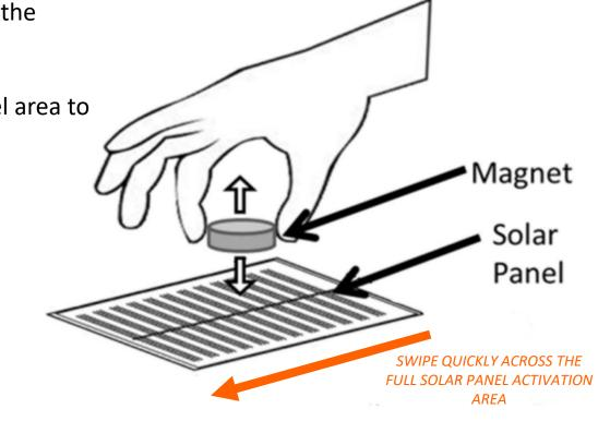
Swipe the included magnet across the Solar Post Cap Solar Panel activation area in full, quick motions to change between the 7-brightness levels, or to place the Solar Post Cap into "OFF" mode.
